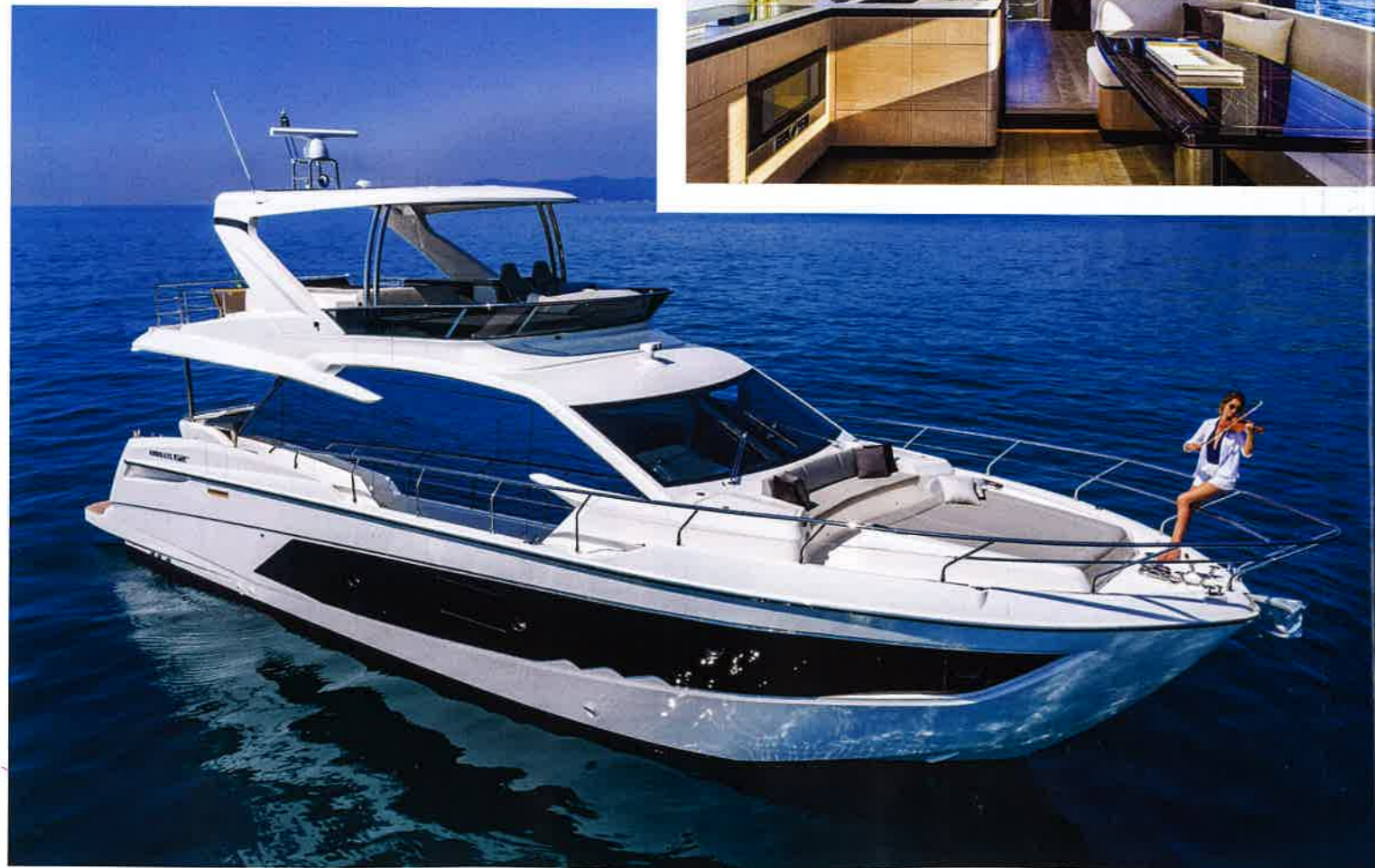
BELOW The 62 Fly is one model in the latest generation of Absolute flybridge yachts. Volvo Penta IPS950 engines ensure smooth, efficient cruising and a top speed of more than 30 knots
