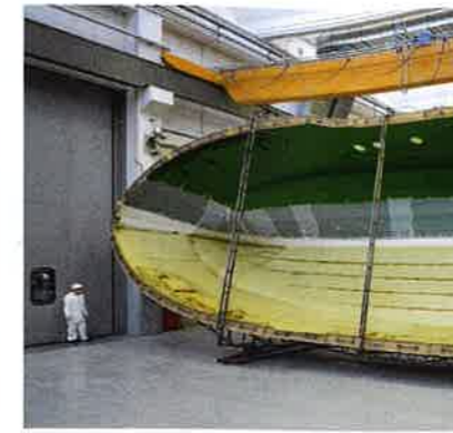
ABOVE LEFT The design process is collaborative with feedback from customers and dealers being passed back to board members, designers and engineers ABOVE MIDDLE A hull mould is flipped inside the construction facility ABOVE RIGHT Two Navetta models await the next stage of their production journey
