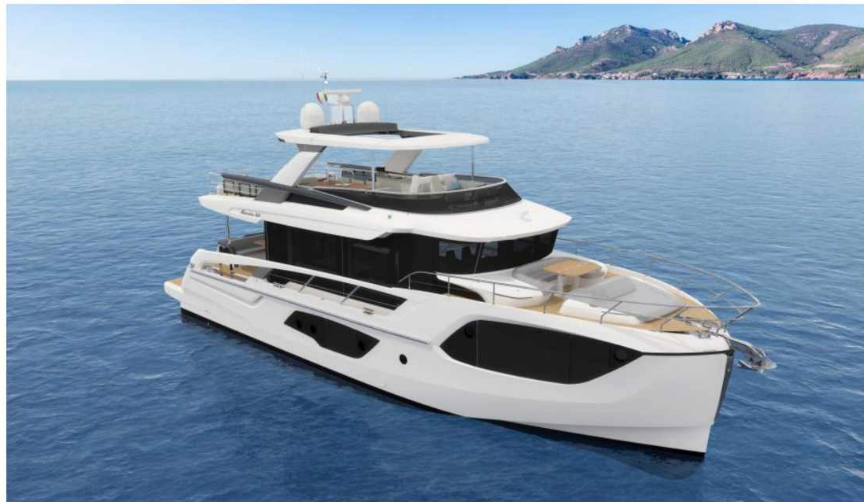
Cutouts in the bulwarks is a new feature on the exterior of the latest Navetta model
