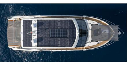
The opening sun roof has been replaced by a set of solar panels on the 48 Coupe.
