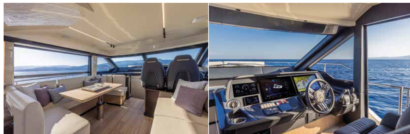
The saloon has a full C-shaped sofa and a facing two-seat sofa behind the twin-seat helm, which benefits from the breeze and access offered by a side door
