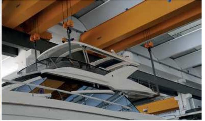
*The bodywork department (left); the superstructure of a 60 Fly (right) is prepared to be lowered onto the hull; an Absolute Navetta 48 in the test pool (bottom)*
