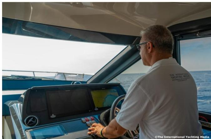
We accelerate a little more and, finally, we reach the cruising speed, that is 22 knots at 3,400 rpm with an overall fuel consumption of just 7 liters per nautical mile. These consumption levels are not bad, especially considering that the l/nm consumption continues to decrease with increasing speed.
