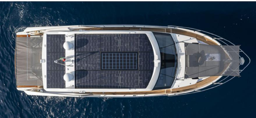
The opening sun roof has been replaced by a set of solar panels on the 48 Coupe.
